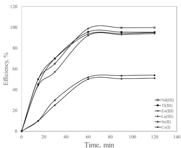
Figure 5. Influence of the contact time on the separation efficiency of the adsorption process
