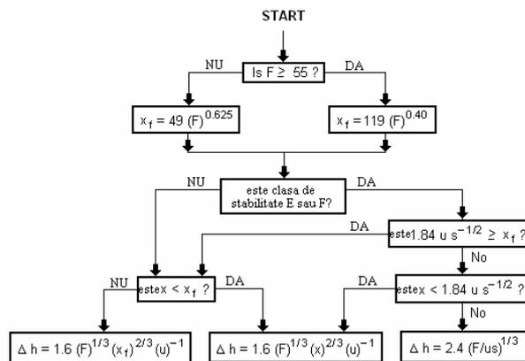
Figure 2 Logical diagram with the calculus algorithm of height of the pollutant cloud
