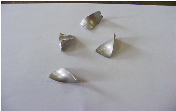
Figure 2. Helical elements as turbulence promoters
