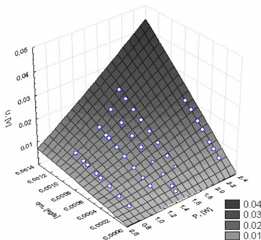
Figure 4. Dependence of the disequilibrium voltage  $U$  on the gas flow rate  $q_m$  and heating power  $P$
