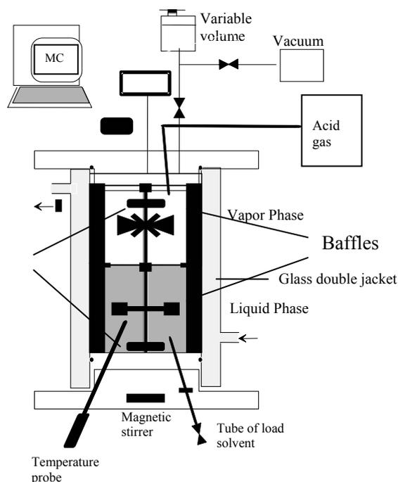
Figure 1. Flow diagram of the absorption equipment
